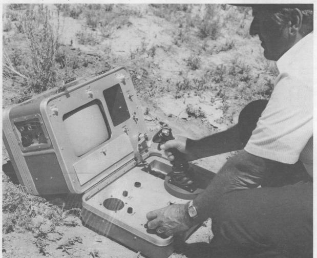
AROD PROJECT LEADER Duane Arlowe (DMTS, 5261) checks out the ground control unit. The portable unit transmits flight instructions to AROD and pan/tilt instructions to AROD's two television cameras. Live TV pictures taken by the cameras are displayed on the 9-in. screen. Larry Fox and Barry Schoeneman (both 5261) did most of the development work on the ground control unit.
